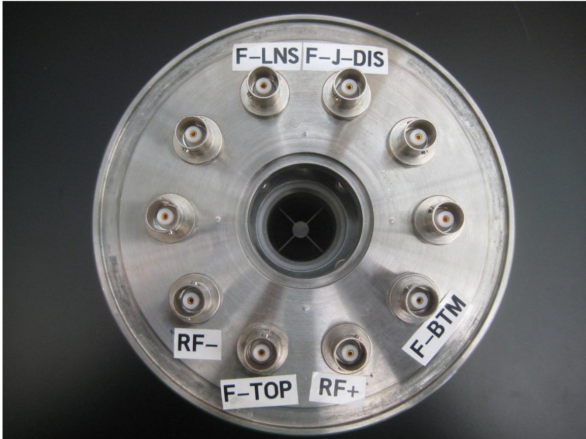
Figure 13: View of the funnel along the axial direction with the heater block/capillary assembly removed. The jet disruptor is clearly visible in the center of the funnel. Also visible are the BNC connectors used to supply the various voltages to the device.
